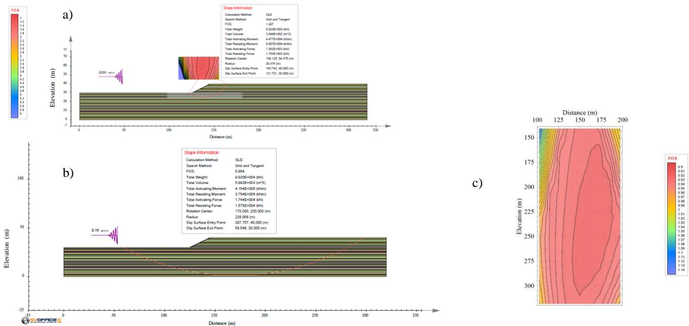
Figure 6: LE simulations carried out for 2H:1V slope angle, slope height of 10 m, deposit thickness of 30 m and increasing shear strength of 1.5 kPa/m a) spectral pseudo-static approach b) conventional pseudo-static approach c) corresponding grid
