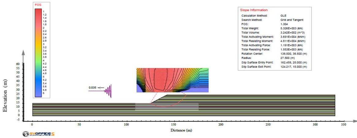
Figure 4: Slip surface for homogeneous clayey slope of 1.75H:1V slope angle, with increasing shear strength of 1.5 kPa/m from the surface to the bedrock. Initial shear strength is of 25 kPa. Slope height is 10 m and deposit thickness is of 15 m.
