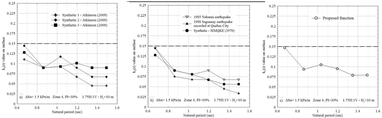
Figure 3: Variation of the proposed spectral pseudo-static coefficient with consideration of frequency content (a) Synthetic-1 – Atkinson [15], Synthetic-2 – Atkinson [15], Synthetic-3 - Atkinson [15] b) 1985 Nahanni earthquake, 1988 [16] Saguenay earthquake recorded at Quebec City [17] and Synthetic – SIMQKE [18] c) proposed function. From Mole et al. [13]
