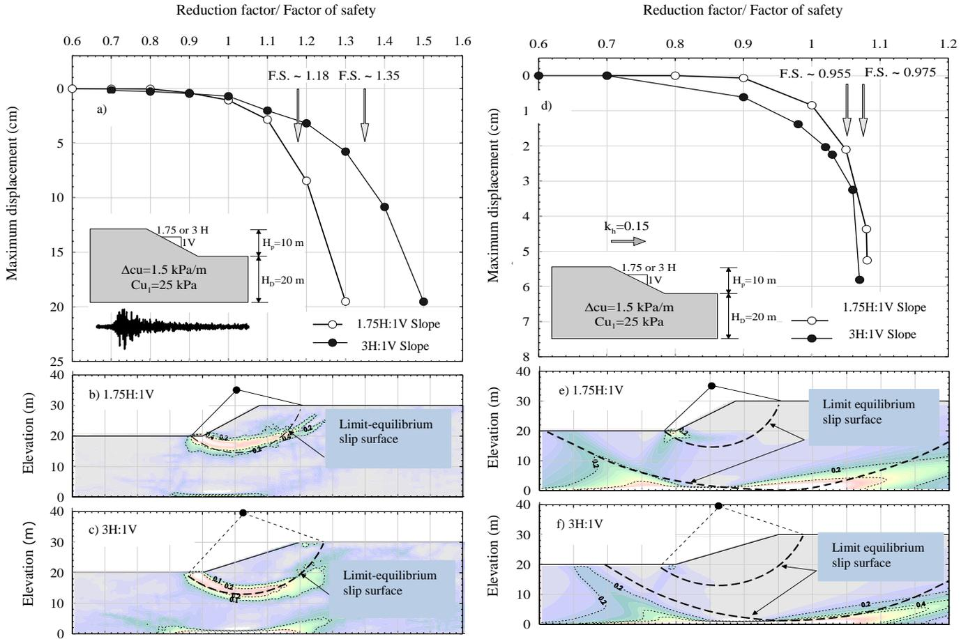
Figure 1: Comparison between dynamic analysis and failure surface obtained using constant seismic coefficient  $k_h=0.15$  as proposed by the Centre d'expertise Hydrique [12] for seismic Zone 4. Dynamic analysis: a) relative displacement-factor of safety curves; slip surface of slope angles: (b) 1.75H: 1V and (c) 3H: 1V. Pseudo-static analysis: (d) relative displacement-factor of safety curves; slip surfaces of slope angles: (e) 1.75H: 1V and (f) 3H: 1V. Adapted from Karray et al. [9]
